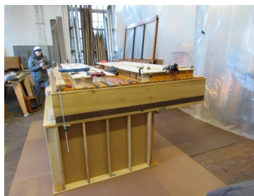
AT RIGHT, THE MAIN WINDCHEST IS BEING MATED TO ITS REGULATED WINDBOX BELOW
