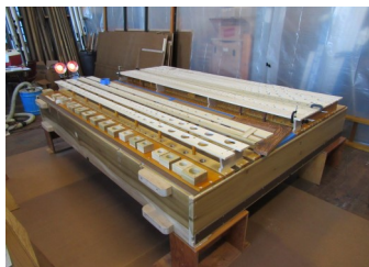
AT LEFT, ALL RACKBOARDS HAVE BEEN FITTED TO THE MAIN WINDCHEST
