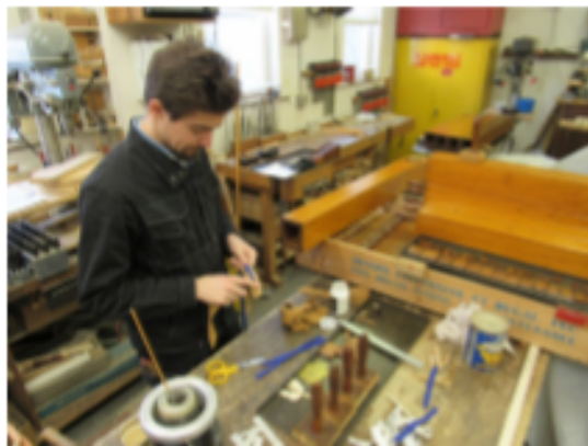
Josh repacked and fitted tuning stops for the Gedeckt 8' pipes.
